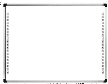
**TDD-IW-IR (Infrared)** Interactive Whiteboard has **infrared** transmitters and receivers, which linked to a USB main board and fixed inside rigid aluminum frames, forming a square scanning infrared ray net on the surface when connected to a computer by USB cable. When a finger or other non-transparent object touches on the surface, this touching point's coordinate (x, y) is immediately transmit to the main board and forms a corresponding PC operation.
